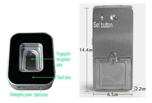
1. Register fingerprint: Insert fine needle(e.g.: clip) into small hole, press shortly set button touched by fine needle, then panel indicator lighten and hearing music, press two times for fingerprint, fingerprint register successful when hearing music. Fingerprint can be registered continuously.
